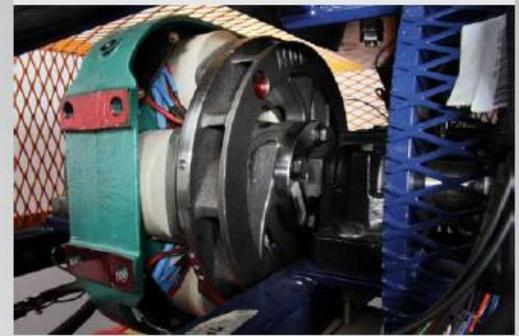
Integrated eddy current dynamometer to vary engine load
